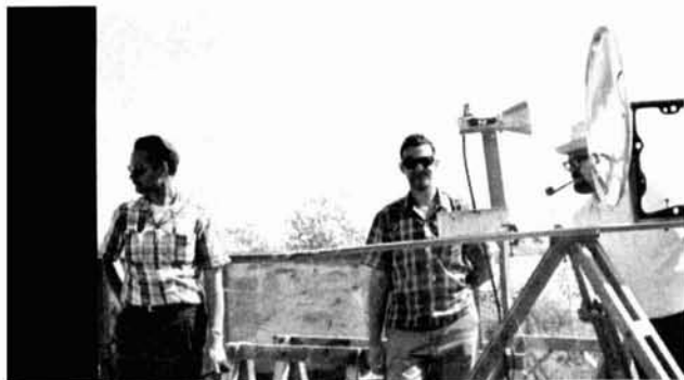
The "Saucer Sled" antenna is being bore-sighted by K6HIJ on a home-brew antenna range. W6DSL and WA6HWV look on.
